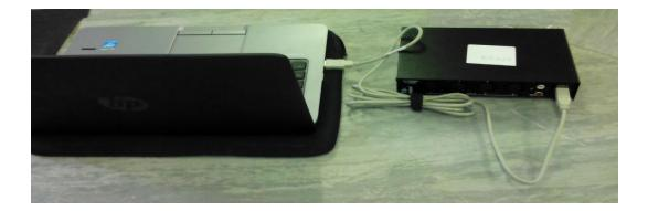
Note: The USB lead must be plugged in and the mixer powered on with Green indicator on front of the mixer before turning PC on.
