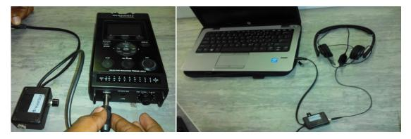
Connect the **large plug** to the Marantz whilst the **smaller plug** is connected in to the **Laptop audio port.** The **headset** is then connected to the **voice box**.
