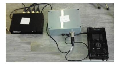
Note: Make sure when you plug in the mixer power the indicator on the front of the mixer is Green. This indicates full power. A Red indicator means low power. To fix this, unplug the power to the mixer and re-plug.
