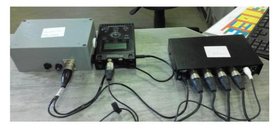
The **red or white** lead should match the **red or white** input port on the **Mixer**. The large lead is connected to the **Marantz** input port that is stating **MONO** on the left side as depicted in the above image.
